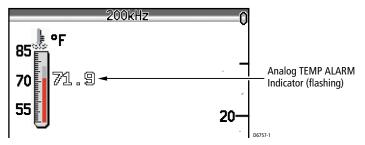
Figure 6-3: Temperature Alarm with Analog Display
